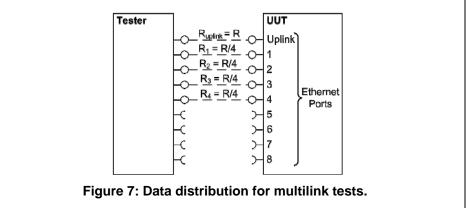
Half port test case shown. R is the rate specified in the procedure.
