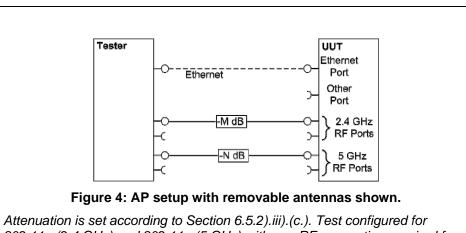
802.11g (2.4 GHz) and 802.11a (5 GHz) with one RF connection required for each to achieve maximum throughput.
