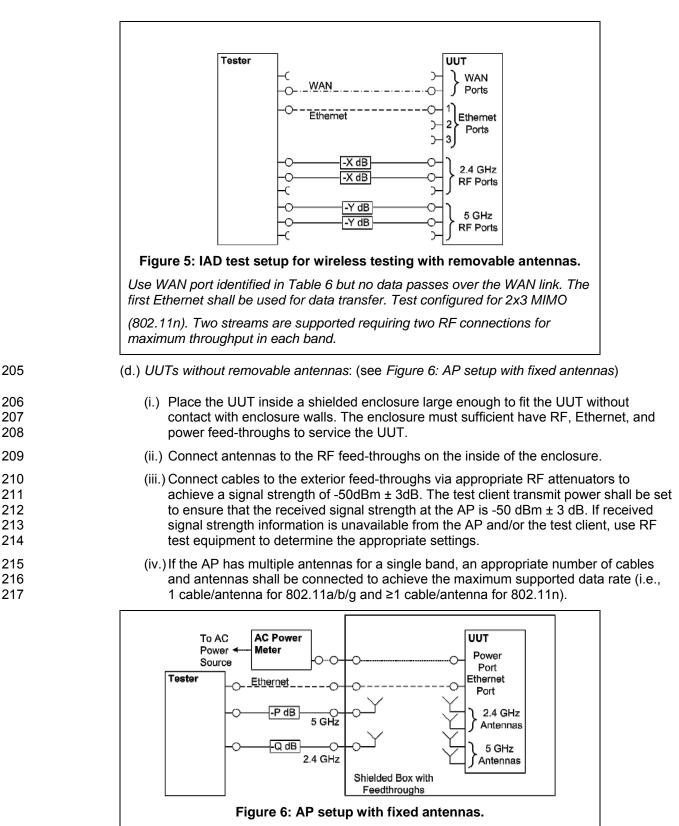
Attenuation is set according to Section 6.5.2).iii).(d.). Test configured for 802.11g (2.4 GHz) and 802.11a (5 GHz) with one antenna connection required for each to achieve maximum throughput.
