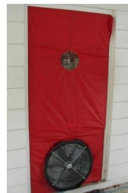
The one exception-where there would be an infiltration limit-is the alternative compliance path to high-performance insulation under item 3.1.2 of the Rater Design Review Checklist (Rater-D). This lesser-used option allows less insulation in exchange for a very tight infiltration rate.
